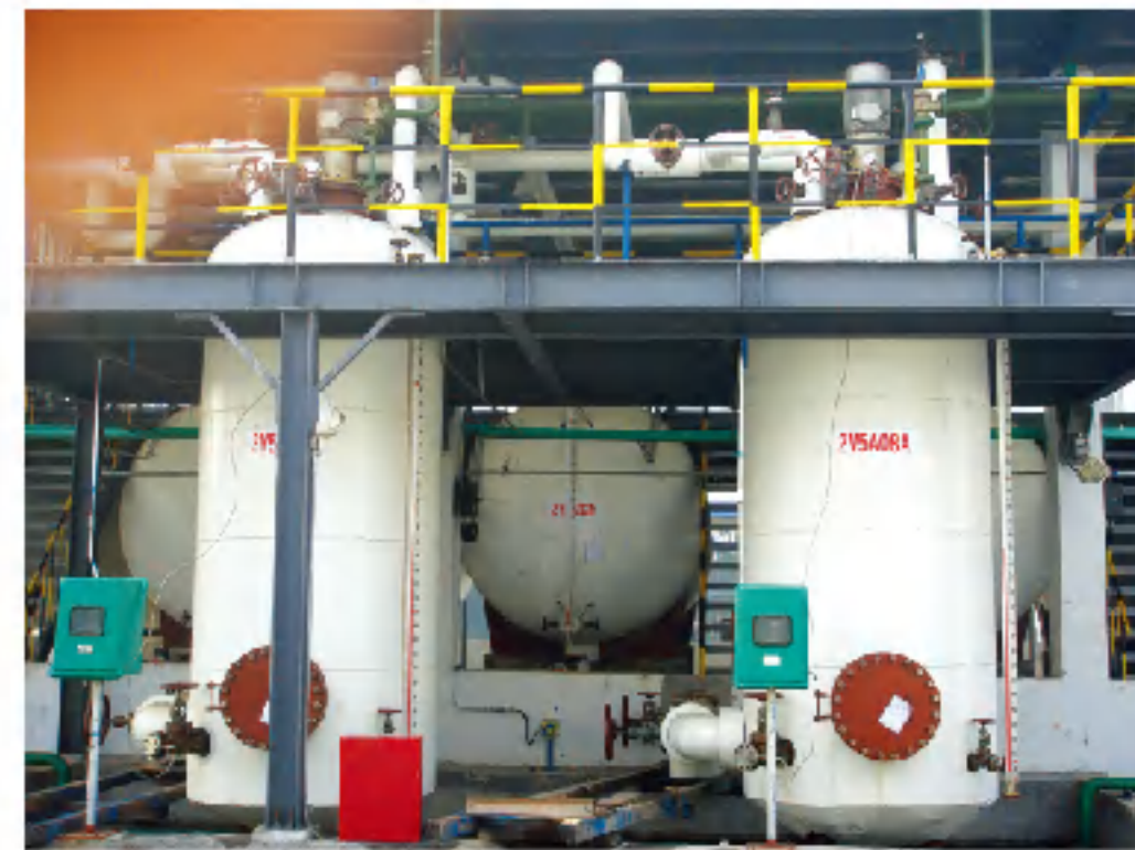
长轴液下磁力泵 Long axis submerged magnetic pump 液下长8米 Submerged Axis length is 8m
