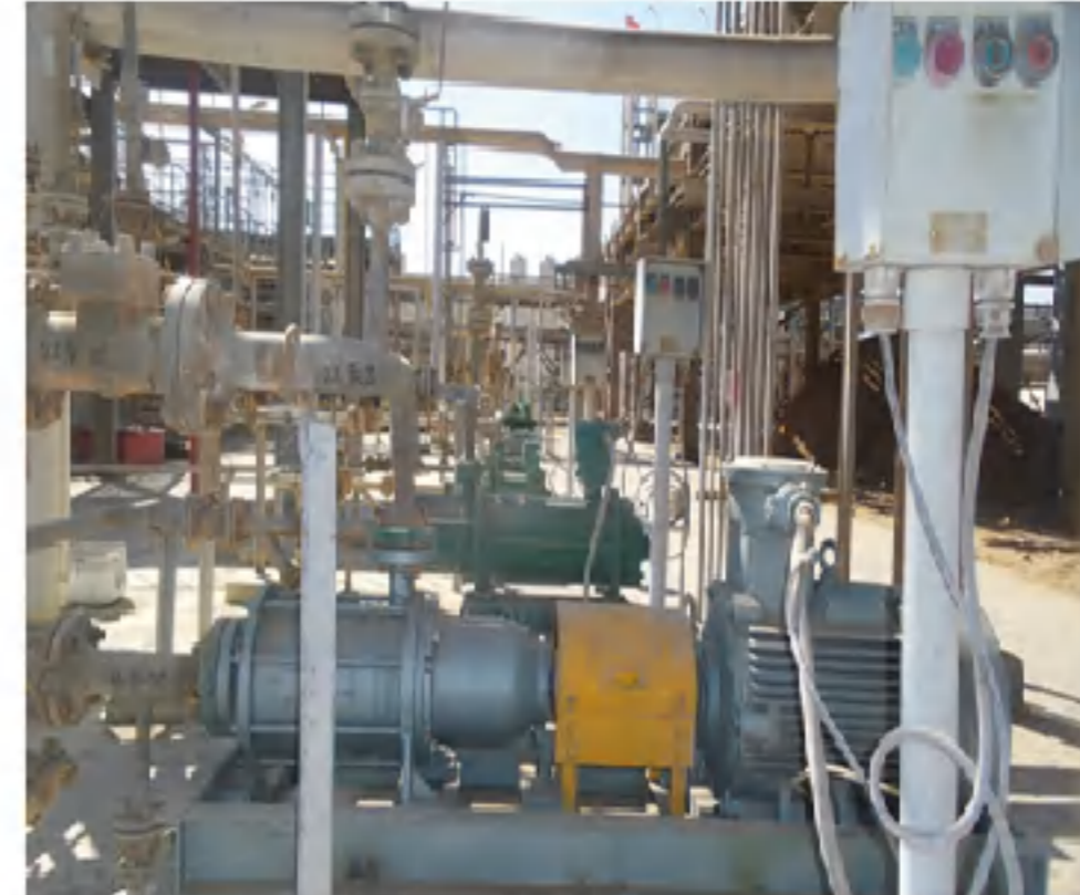
多晶硅冷氢化装置 三氯氢硅输送泵 Pump for SiHCl 3 in Polysilicon cold hydrogenation unit
